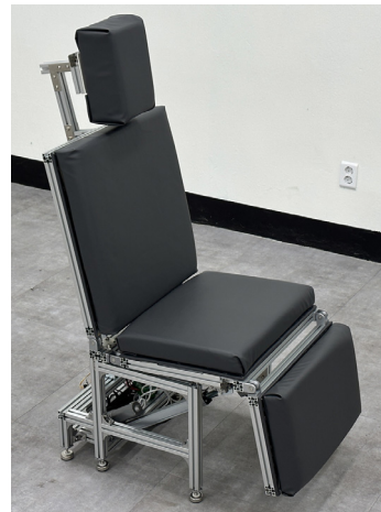
Fig. 8 Manufactured experimental seat model
